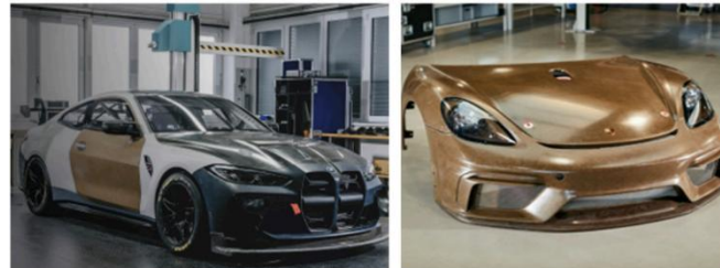
Figure 7. Composite parts fabricated using different natural fibres (a) Generalized history adapted from 95, (b) BMW iFE.20,9% and (c) Porsche 718 Cayman GT4 Clubsport.
